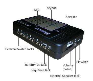
Note: The battery cover is located on the bottom of the Medley.
